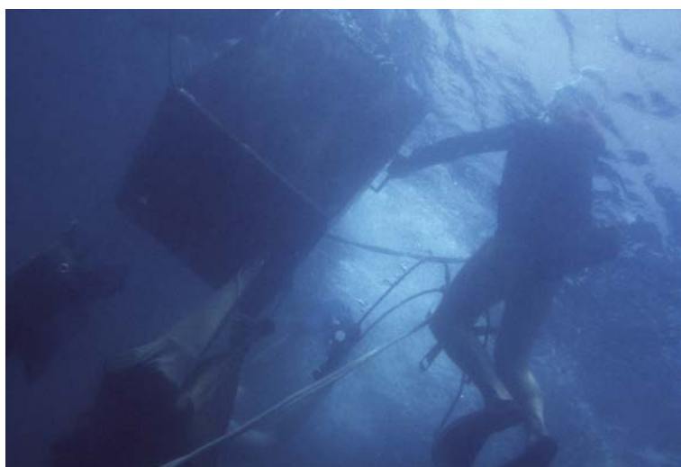
Fig. 12. Keeping the bell's buoyancy under control proved quite difficult – lead weights which were loaded into jute sacks had to be used to compensate it; Photo by Andreas HANTSCHK & Peter ELSTER.
